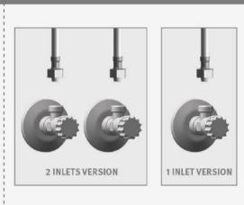
MAKE SURE THAT THE FILTER(S) IS/ARE INSTALLED BETWEEN THE FLEXIBLE PIPE AND THE SHUT OFF VALVE (ANGLE VALVE) (NOT SUPPLIED).
